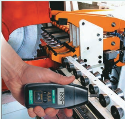
Accessory wheels enable tachometer to measure linear speed surfaces
