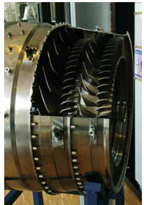
The turbine wheel (MTU Aero Engines GmbH) consists of a heavy, high-strength nickel alloy.
