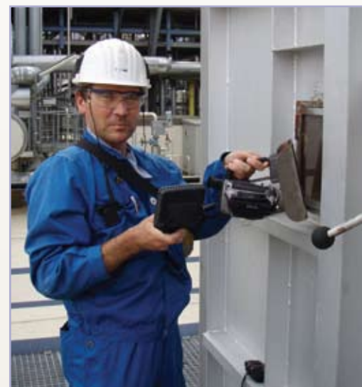
Holger Springer with his FLIR infrared camera at a furnace inspection window
