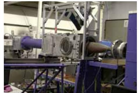
*The air flows from the pressure chamber (to the right) through the test chamber (middle) and into the vacuum tanks (left), reaching air speeds of over 4000 kilometer per hour.*
