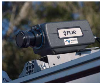
FLIR A6701sc camera used to create infrared delamination maps
