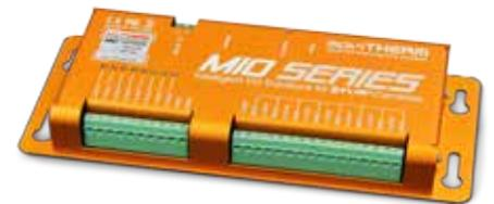
The MoviTHERM MIO (Intelligent I/O) module provides discrete electrical connections needed to generate alarms and warnings based on predefined temperature conditions.
