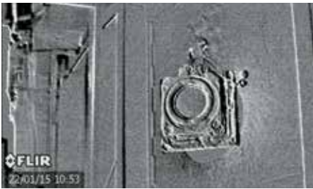
A FLIR GF306 can easily detect ammonia gases escaping from a gas nitriding furnace.
