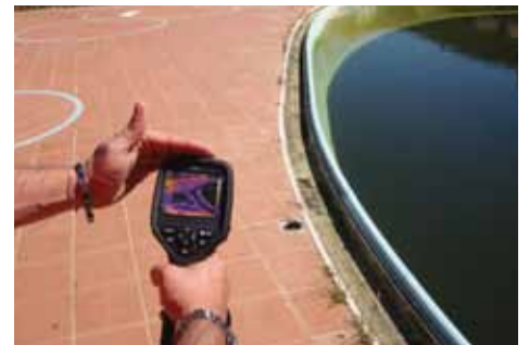
The FLIR E60 thermal imaging camera clearly localized the water leaks.
